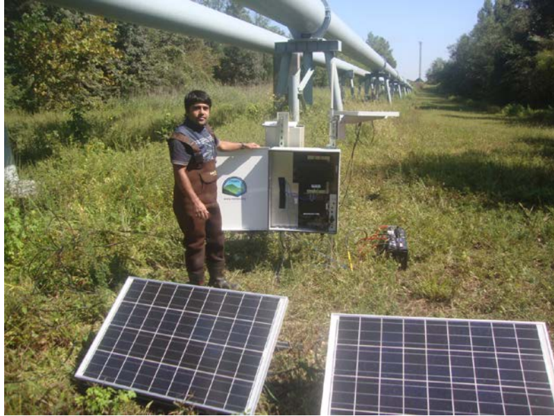
Figure 2.6. Distributed temperature sensing (DTS) equipment deployed in the field in Sept. – Oct. 2011.
