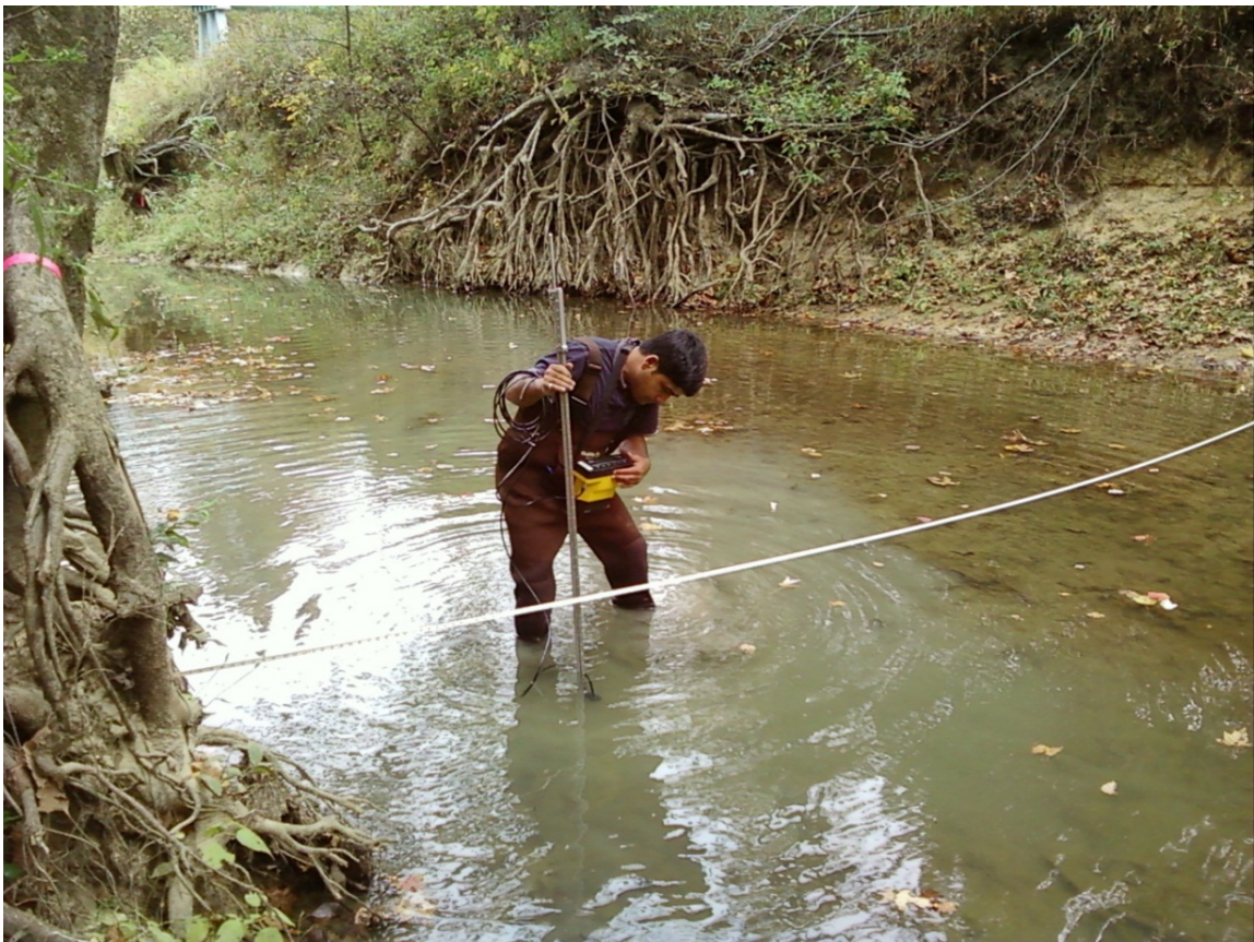
Figure 2.1. Stream gauging in October 2010 along transect EB2U, upstream of farthest downstream spring EB2, which is located behind exposed roots on far bank.
