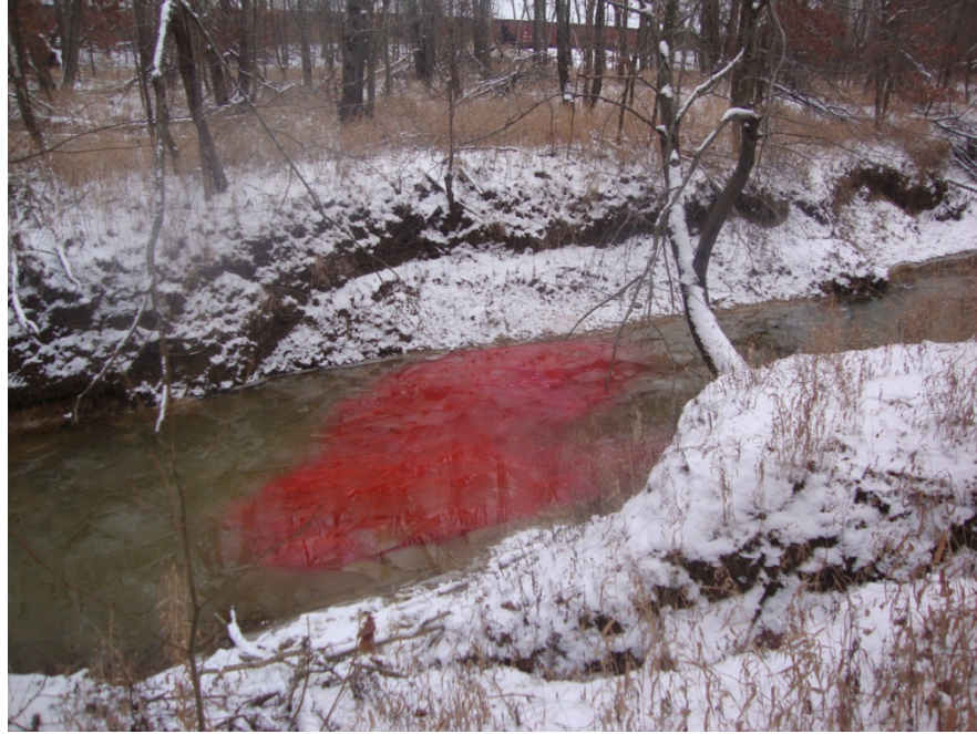
Figure 2.2. Rhodamine WT dye cloud moving downstream. Photograph taken in January 2011 during dye dilution tracer test.
