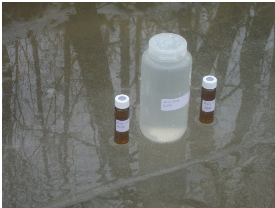
Figure 2.3. Sample collected for VOCs and ^{99}\text{Tc} analyses in January 2011. Samples resting over the ice sheet on top of the stream surface.
